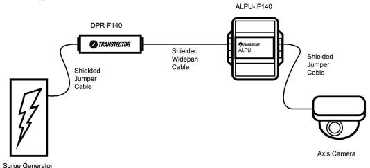
The Transtector PoE solution was lab tested using a surge generator, shielded mid-span cable, surveillance camera, and (2) Transtector hybrid design data SPDs (DPR-F140) and (ALPU-F140), the diagram below reflects the test configuration. Using the surge generator, the camera was hit with (18) 1KA surge events. After the test conditions were applied, the camera produced crystal-clear images, which proved operational status after multiple surge hits.
