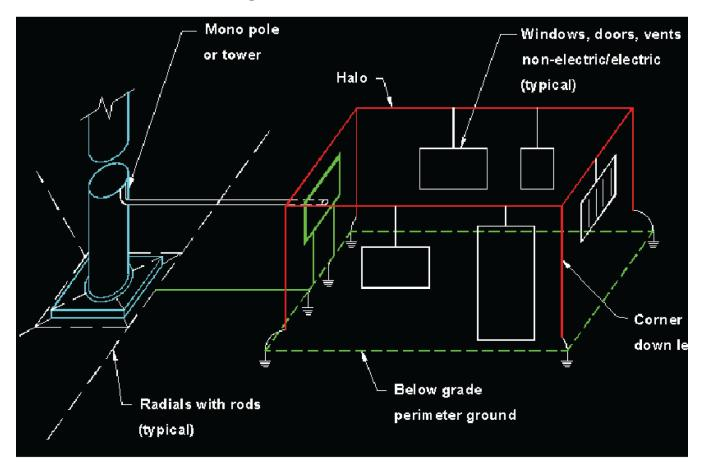
(1) The halo should not be interconnected with or used as a ground connection for any active electronic equipment. Do not attach the halo to the single point ground, equipment racks or the entrance panel / bulkhead / hatchplate / coax line ground bar.
