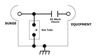
The IS-50/B50 series products are capacitive coupled gas tube protectors with multi-strike capability. As DC block products, they do not provide continuity from center-pin to center-pin, or from center-pin to shield. Low frequency surge current induced onto the center-pin from the antenna side is blocked by the capacitor until the gas tube reaches its "turn-on" voltage to shunt the surge to ground (assuming the IS-50/B50 unit is properly grounded).
