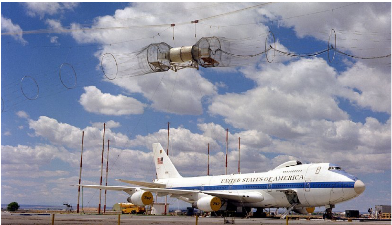
EMP simulator HAGII-C testing a Boeing E-4 aircraft. US DoD, Wikimedia Commons.
