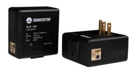
The SLN 120 AC surge protector is a solid-state SASD (Silicon Avalanche Suppressor Diode) device designed to protect electronic equipment and systems from transient over voltages on 120 Vac single phase services. The SLN 120 offers continuous bi-polar, bi-directional protection, with the ability to automatically reset after each suppression function with no degradation of protection capabilities.
