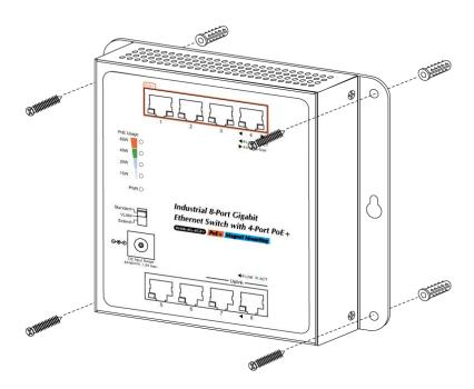
**Step 2-2:** Or the Switch, as shown in the picture below, can be hung on the wall by screwing the two screws leaving a space of 2mm apart after the anchors are hammered in.
