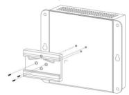
Step 2: Lightly press the bottom of DIN-rail bracket into the track.
