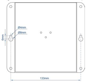
**Step 2-1:** Hammer the anchors provided into the four holes and use the four screws to tightly fix the switch onto the wall by screwing them in.
