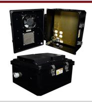
temperature set point accuracy. The fan turns on when the internal temperature rises to 90° F (32° C) ±5° and turns off at 81° F (27° C) ±5°. The cooling fan does not require the use of any of the AC outlets, leaving them all available for your equipment.
